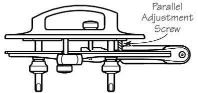
**Figure 5: Parallel adjustment (bottom view).**
