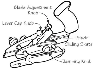
**Figure 4: Blade installation.**
