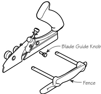
**Figure 2: Preparing the small plow plane.**
