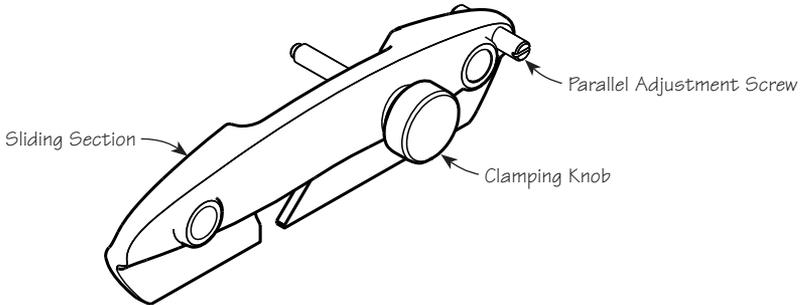
**Figure 1: Conversion kit components (right-hand version shown).**
